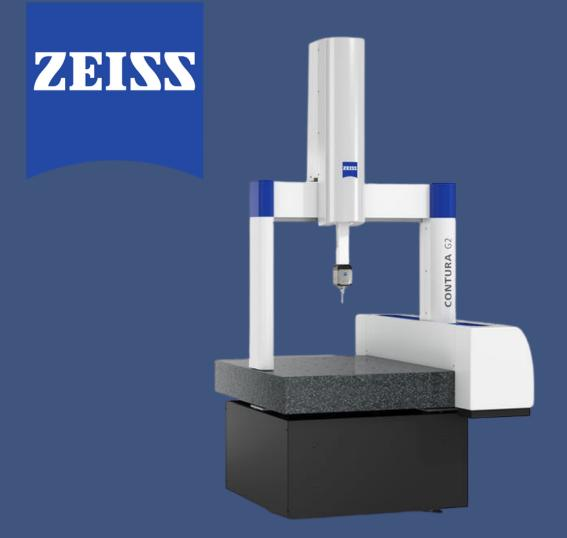
Carat guideways are used on Zeiss Contura for high rigidity, low thermal expansion and minimal moving weights. Air bearings in all three axes ensure consistent stability even at high travel speeds and acceleration.
