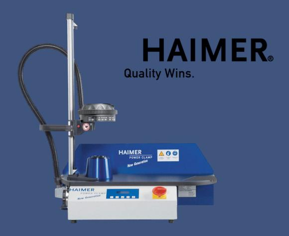
Shrink fit chucks grip the cutting tool 360° around the shank on multiple planes, delivering very high gripping torque that prevents chatter during roughing or finishing operations.
